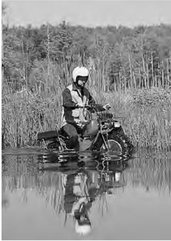
The ROKON can be used to cross slow moving shallow water of up to a maximum of 24 inches in depth. Before entering the water, choose your path carefully. Enter where there is no sharp drop off, and avoid rocks or other obstacles which may be slippery or upset the ROKON. Drive slowly and carefully. Never change your course in the middle of a stream or you will find that slippery rocks and currents might throw you out of balance.
