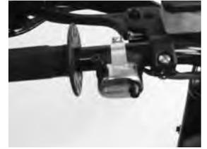
**Fuel Tank Shut-Off Valve:** Located on the right hand side under the fuel tank shuts off fuel flow to the engine. The down position is for fuel flow. The up position shuts fuel off. Shut the fuel off when storing or transporting your ROKON.
