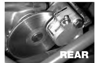
**Choke:** Choke is used to start a cold engine and should be in the rearward position to choke. It is located on the right hand side of the engine. As soon as the engine starts, the choke should gradually be moved forward as the engine warms up. It should be left fully forward for regular operation.
