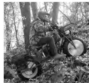
When riding downhill, shift your weight as far to the rear and uphill side as possible. Use low gear and engage the throttle slightly to allow the engine compression to provide braking. Whenever possible ride straight downhill. Turn into corners with the rear brake only, so as not to slide the front wheel and lose steering control.
