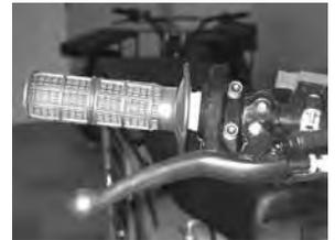
**Brakes:** The ROKON is equipped with separate front and rear disc brakes. The left brake lever is for the rear brake. The right brake lever is for the front brake.
