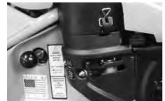
**Engine Fuel Valve:** Located below the choke. Valve should be in rearward position when bike is not being used. Valve should be moved to forward position for use. Close when storing or transporting your ROKON.
