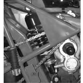
**Rider Seat Suspension:** The seat suspension spring can be adjusted to suit the rider's weight and riding conditions. Adjust the spring per load as follows: To increase the spring preload, turn the adjuster clockwise. To decrease the spring preload, turn the adjuster counterclockwise.
