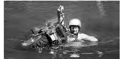
If the water is over 24" in depth, shut the bike off and always float your machine across (hollow wheels only). Keep the air intake out of the water to avoid flooding the engine compartment by always floating the bike with the right hand side above water (as shown in picture on right).
