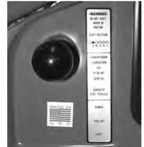
**Automatic Torque Converter:** The torque converter is designed especially for ROKON and provides smooth automatic clutching and ratio changing in response to throttle control and terrain requirements. The front driven pulley tends to shift into high as engine speed is increased. The rear driven pulley follows this speed change. If torque requirements increase, the cam in the torque-sensing rear pulley overrides the front pulley and forces a down shift without a loss of engine revs and power.
