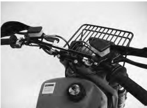
braking with the front brake, the machine should be in a "straight away" position. Hard braking, with a turned front wheel, can cause loss of steering which can result in loss of control. The rear brake (left hand side) should be used more often for going down steep slopes.
