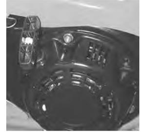
**Recoil Starter:** Firmly grasp the handle and pull slightly until engagement can be felt. Then pull forcefully, being careful not to pull the rope all the way out. Return the starter rope gently.
